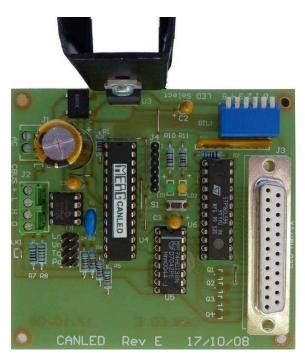
CANLED is a module used to control track indicator LEDs that form a mimic panel or display.
