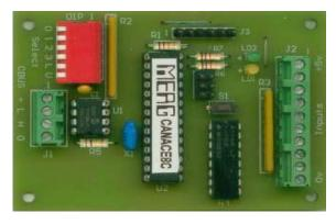
**CANACE8C** is a module that is used to input signals that are processed by the system to provide information about layout accessories. E.g. this module can be connected via micro switches to test the position of a turnout.
