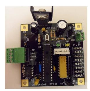
**CANSERVO8** is a module to control low cost servos like the Tower Pro SG90. Typically, these units will operate turnouts, semaphore signals, road crossing gates and other moving layout features. The SG90 can be purchased on EBay for less than AUS\$5.00 [about £3.00] and when mated with moving accessories, it can be a versatile combination for an economical price.
