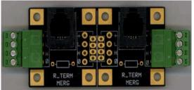
CAN-RJ22 module is used to interconnect CBUS layout wiring to the CANCAB module. It uses a standard telephone 'curly cord' cable with RJ22 type connectors to connect to the handset controller. Convenience and practicality
