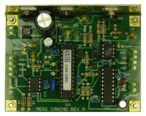
**CANCMD** is a module connected to CBUS and is controlled by the CANCAB handset or the JMRI throttle screen. It creates and sends the DCC signals to the track via the NB1B booster. If less than 1 amp DC track power is required, it can power the track directly without the need of a booster.
