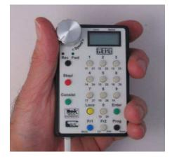
**CANCAB** is a small hand held module that controls a loco's speed and direction; in addition it can also operate turnouts and other moving layout accessories.
