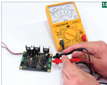
Testing starts by connecting the board to a 16V AC feed. The voltage is checked at several points using a multimeter and the regulators checked for excess heat.
