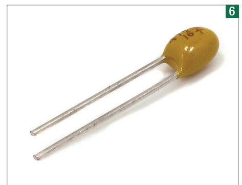
Where polarity matters, identify the + and - sides of a component. Tantalum capacitors like this have different length leads, the longest being positive.
