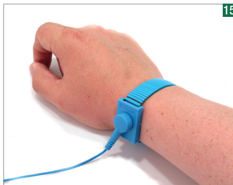
The chips can be damaged by static electricity so earth yourself by wearing an anti-static wristband clipped to a nearby water pipe before handling them.
