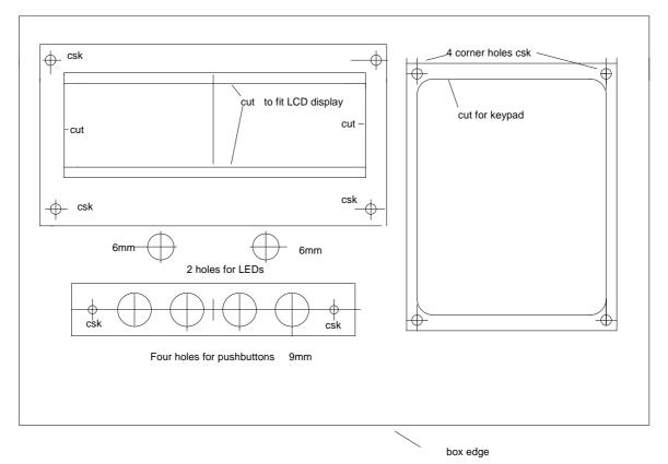
The small screws can be M2, M2.5 or 8BA. countersunk
