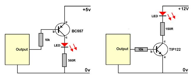
The one on the left uses a transistor as a switch for currents up to 100mA, the maximum that the transistor can handle.
