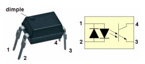
transistor and switches it on. Current can now conduct between its output pins.
