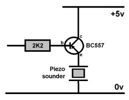
If your module's output can handle that amount of current, you can connect the buzzer directly to the output pin. When a DC voltage is applied across it, it will emit a continuous high pitched tone.
