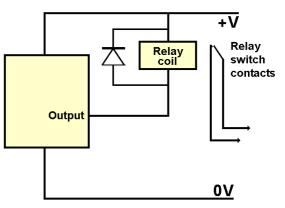
If there is any doubt about the above circuit, you can check what the module's current handling capacity is and compare it with that need to operate your relay. If you are lucky, you will have the relay's specification which will include its coil resistance, allowing you to calculate the expected current for the supply voltage you are using.
