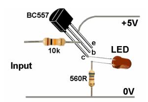
If you intend to illuminate a very high power LED or a LED strip that contains multiple LEDs, you need to use a transistor that can handle these larger currents.
