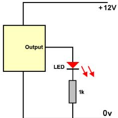
This illustration shows the LED being wired to 0V. In this case, the LED will illuminate when the module's output pin goes high.
