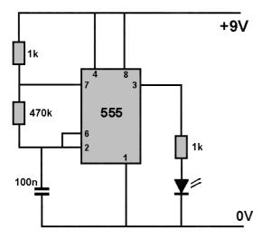
Because we can vary the mark/space ratio, we can create circuits where the 555 lights a LED with a 50/50 ratio or just lights it for a short time every so often.
