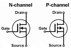
emitter current to control output current, the FET has almost no gate-source current flow. Applying a voltage to the gate generates an electrical field and this controls the current flow through the channel between the source and the drain.
