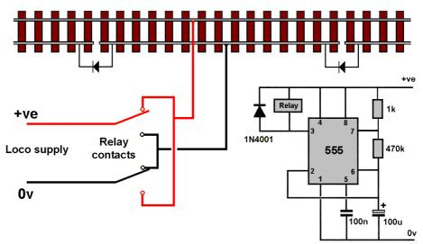
You can apply formulae to calculate the frequency and also the mark/space ratio for any given set of components.
