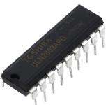
The other pins are arranged in pairs with the input pin facing across from the output pin. So, pin1 is the input pin that controls output pin 18, pin 2 controls output pin 17 and so on.
