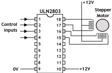
Here is an example of controlling a motor. When pin 3 goes high, pin 16 goes low and the motor turns.
