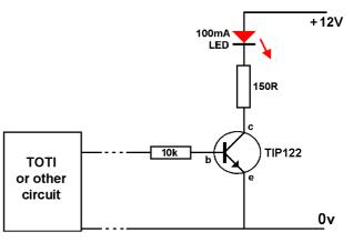
used to produce the TIP122's base-emitter current. Once again, the smaller base-emitter current results in a much greater collector-emitter current.
