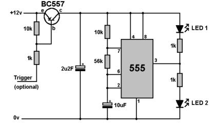
This continually repeats, at a rate set by 10uF capacitor and the 10k and 56k resistors.
