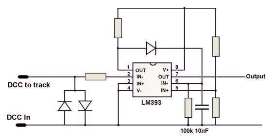
Pin 4 is permanently held at 0V. When a loco enters a section of track, the DCC voltage develops voltages pulses across the diodes and this is passed to pin 2. With every pulse that takes pin 2 high, pin 1 goes low, so there is a constant stream of pulses on pin 1 (as long as the loco remains in that track section).
