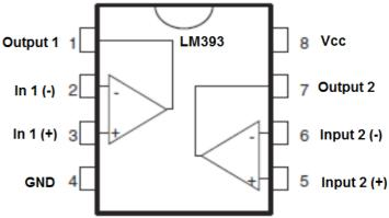
If the voltage at the inverting input is higher than at the non inverting input, the output turns on (i.e. goes low).
