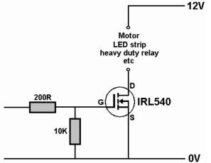
The 200 Ohm resistor is there to protect the attached circuit should the MOSFET fail and to
