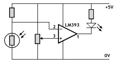
The voltage on input 2 depends on the voltage at the junction of the resistor and the light
