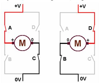
When switches A and C are closed, the motor has a positive potential on its left hand connection and 0v on it other connection. The motor will turn in one direction. If we now open switches A and C, and close switches B and D, the voltage across the motor is reversed and the motor turns in the opposite direction.
