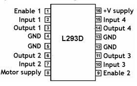
The enable pins can be switched externally, where bringing it down to 0V stops the drivers from working. If this is not needed, the pins can be permanently connected to +5V. They can also be fed with a PWM signal to control the motor speed. See the chapter on Loco Controllers for a description of PWM.
