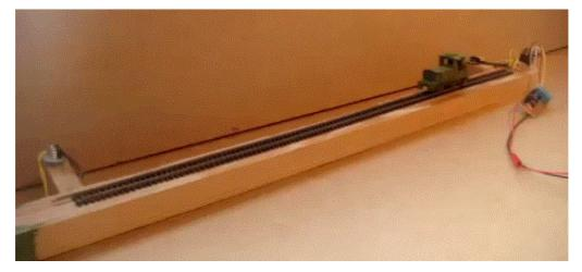
A microswitch is fitted at each end of the track, with extended paddles added so that they span the track.
