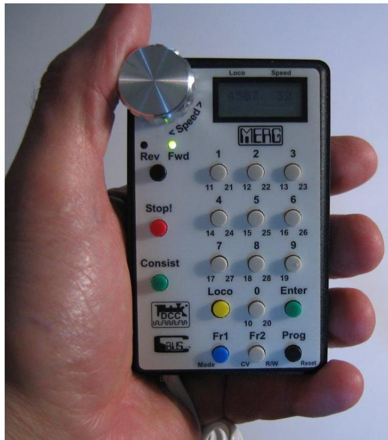
Figure 11. Completed CAB in use.
