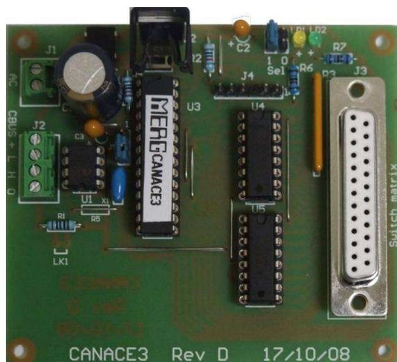
**CANACE3** is a module used by the system to find the status of mimic panel switches. A single switch can operate a single turnout or multiple turnouts and even a complete route. Conversely, more than one switch can control a single turnout or signal. This is similar control that can be configured on a wired relay panel without its wiring complexity. Toggle switches or push buttons are supported by software.
