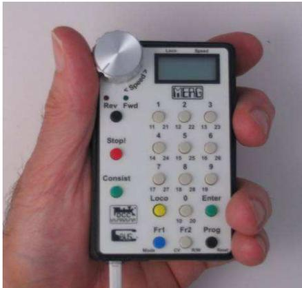
**CANCEAB** is a small hand held module that controls a loco's speed and direction; in addition it can also operate turnouts and other moving layout accessories.
