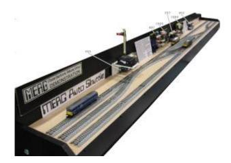
The shuttle module or ATC (Automatic Train Controller) MERG Kit 46, comes preprogrammed with a number of different configurations, selectable using an on board 4 way DIL switch. The track on this demonstration board is a symetrical arrangement that allows all of these configurations and the module cycles through these.
