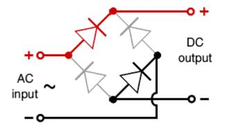
The diagram shows the operation of a bridge rectifier as it converts AC to DC. Notice how alternate pairs of diodes conduct.
