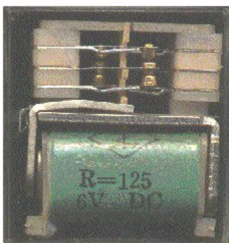
Relay showing coil and switch contacts
