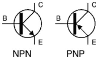
The leads are labelled base (B), collector (C) and emitter (E). These terms refer to the internal operation of a transistor but they are not much help in understanding how a transistor is used, so just treat them as labels!
