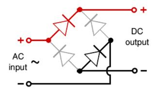
The diagram shows the operation of a bridge rectifier as it converts AC to DC. Notice how alternate pairs of diodes conduct.
