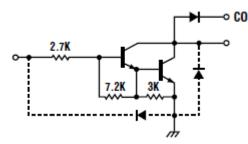
In electronics, the Darlington transistor is a semiconductor device which combines two bipolar transistors in tandem (often called a "Darlington pair") in a single device so that the current amplified by the first is amplified further by the
