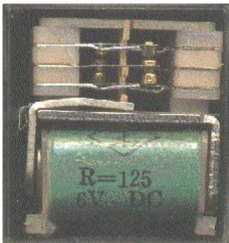
Relay showing coil and switch contacts
