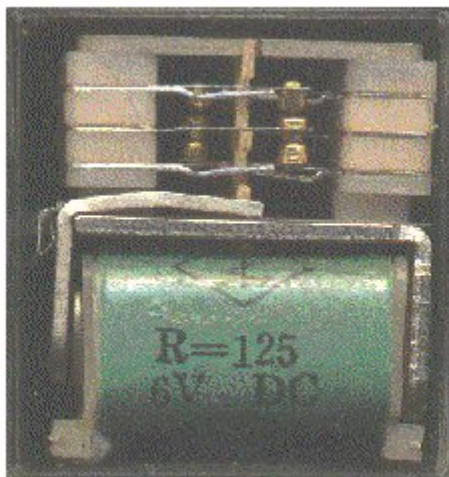
Relay showing coil and switch contacts
