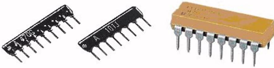
“Resnets” come in 3 basic package types. Pin at one end is common to all (odd number of pins). Individual resistors in single line, pair of pins for each resistor. Individual resistors in DIL, resistors connect to pins on opposite sides of package.
