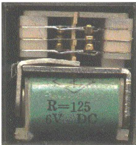
Relay showing coil and switch contacts
