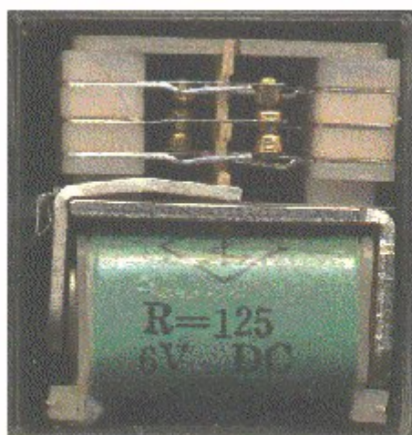
Relay showing coil and switch contacts
