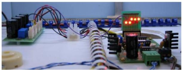
Instead of an LED in the top left position, a wire is taken to a PD3 point motor driver (kit 37a) and this controls both points on the demonstration layout.
