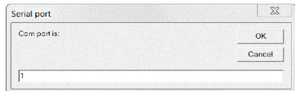
The user can simply try selecting each port number in turn until the application works. In well-written applications, entering the wrong port number simply results in an 'Invalid port number' error message. The experienced user might wish to use Window's Device Manager to examine which COM ports may already be in use.
