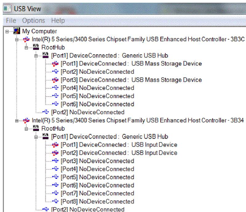
In the example shown, the computer has two host controllers and two root hubs. Two of the ports are used for connecting to memory cards readers built in to the computer, while the other root hub has two input devices (USB mouse and USB keyboard in this example) attached externally.
