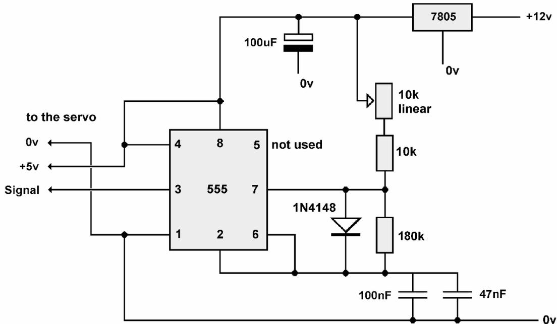
If a pulse is 1mS long, the arm will move fully in one direction, while a 2mS pulse duration rotates the arm fully in the opposite direction, Any pulse width between 1mS and 2mS results in an intermediate position (e.g. a 1.5mS pulse will move the servo arm to mid position).
