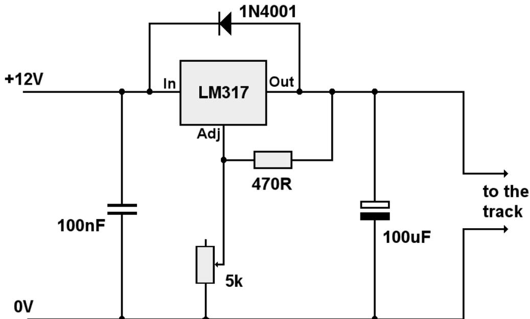
The LM317 is a 3-pin device that can have its output set to provide output voltages from 1.2V upwards (it does not go down to 0V). The output depends on the input fed into it and the combination of the resistor and potentiometer values that provide a voltage feedback to the chip's adjustment pin.
