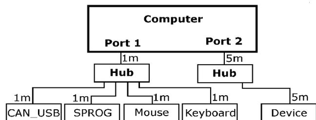
The diagram shows a PC with two USB ports. Port 1 connects directly to a hub and this has four outlets connected to typical USB devices.
