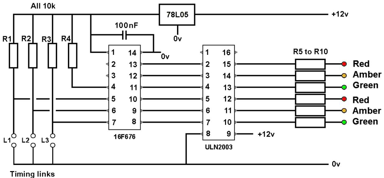
R1, R2 and R3 ensure that pins 5, 6, and 7 on the PIC chip are kept at a high voltage, unless links are wired across to 0V. When a wire link is inserted, it pulls that pin down to 0v. The PIC knows which timing sequence to use, based on which links are made (see table above).
