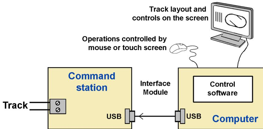
The command station connects to power and to the track as normal. A USB cable is used to connect the command station to the computer.
