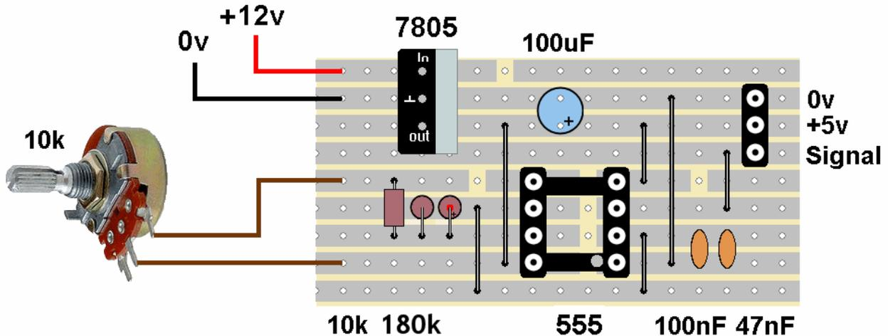
The first step is to cut breaks in the track at the points shown in the illustration.
