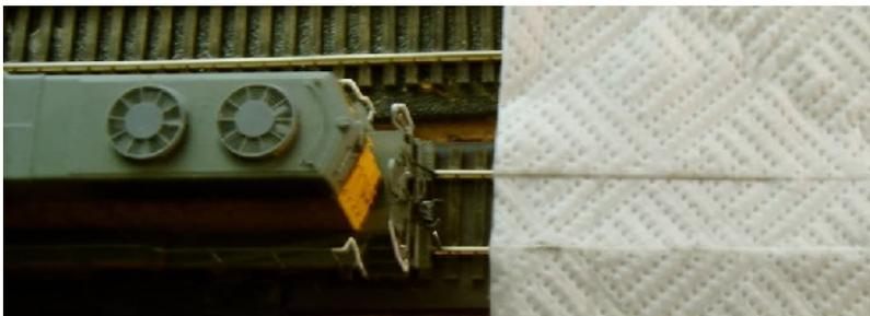
If you prefer not to use abrasive materials, you may consider this simple but effective way to keep wheels clean. A piece of J cloth or paper towel is placed over the track and drops of cleaning fluid such as IPA are sprinkled on the areas that are over the tracks.
