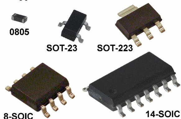
SMD components are so small that it is difficult to print conventional markings on them. Often, they will have no markings and have to be kept in separate plastic bags with labels. They are usually supplied on a bandolier (a 'film strip' with many sealed pockets) and should be kept there until they are ready to be mounted on your modules.
