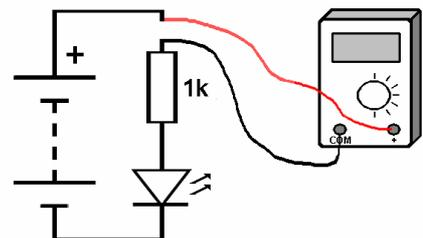
Most often you will be checking the current drawn by an entire module. Here, the multimeter is placed in series with the power lead to the module. Again, observe polarity – i.e. the red lead to the more positive side of the circuit.
