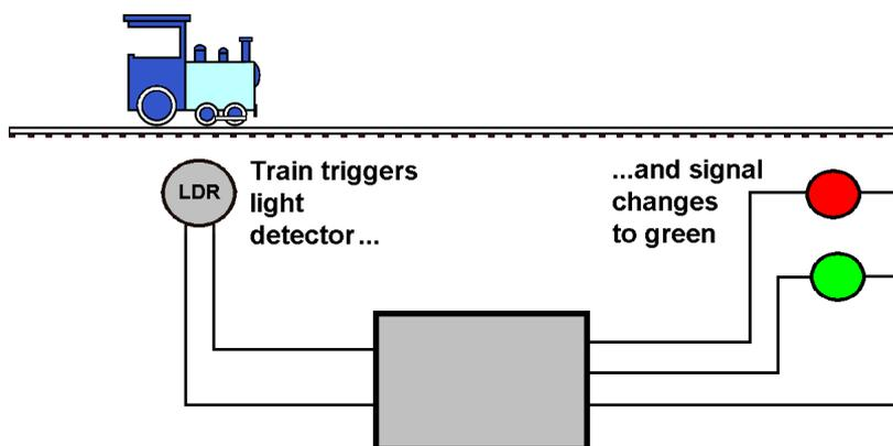
This circuit uses the same detector circuit but blocking the light to the light-dependent resistor (LDR) triggers a timer that is added to the board. This results in a module with a single function but one that is useful and not readily available or at a reasonable price. This illustration shows the setup.
