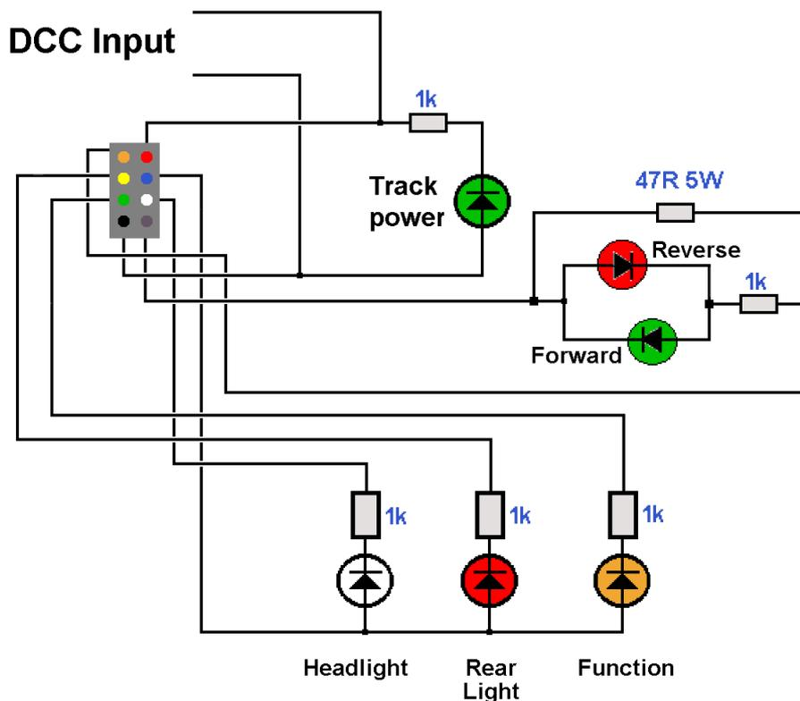
The DCC decoder is plugged into the module's 8-pin socket.
