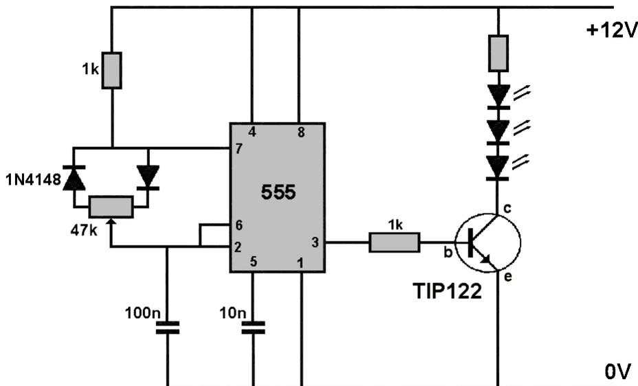
It uses a 555 timer chip which runs at a fixed frequency of a few hundred Herz (i.e. the number of times its output switches between low voltage and high voltage every second). The output from the 555 chip (pin 3) is a square wave that has a variable 'duty cycle' (the time that the voltage is high compared to the time it is zero). The duty cycle can vary from 0% (never on) to 100% (always on) and is determined by the setting of the 47k potentiometer
