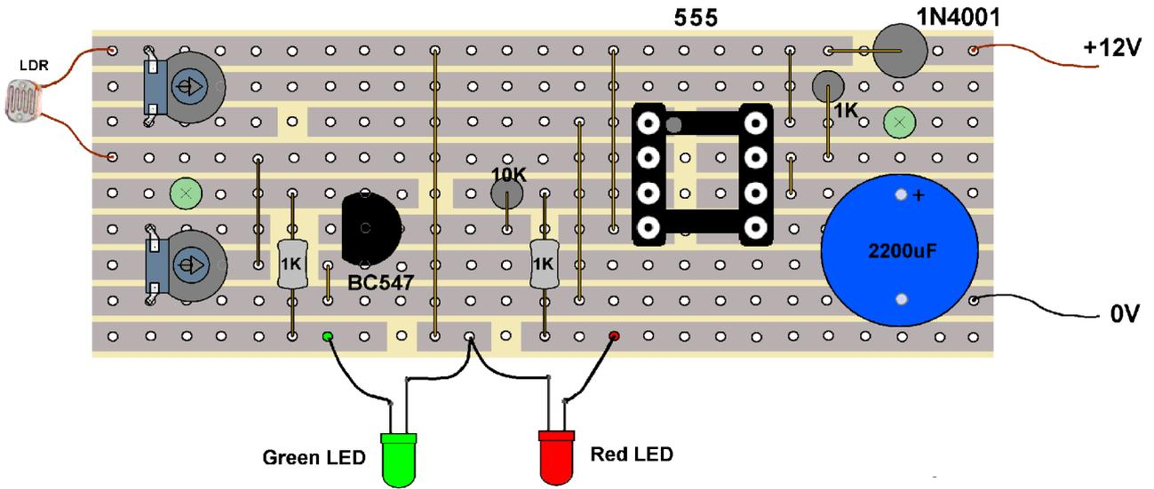
Layout for common anode signals
