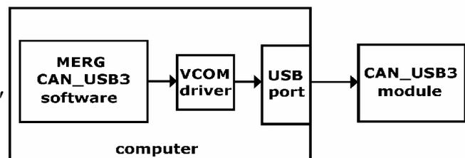
FTDI, the company that manufacture the UM245R USB interface module used on the CAN\_USB3 module, provide an appropriate royalty-free driver (VCOM or VCP- Virtual COM Port) from their website. It is packaged as the *'Combined Driver Model'*. This driver emulates a standard PC serial port, saving program writers from the many complications of handling USB communications.
