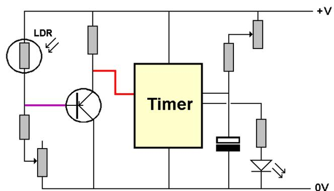
This analogue change of voltage is taken to the transistor – the purple line shows the transistor's analogue interface.
