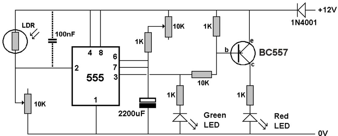
When the loco passes over the LDR, it blocks the light reaching the LDR. In darkness, the LDR has a very high resistance and this lowers the voltage at the junction. The 10k trimmer is used to adjust the sensitivity of the detector.
