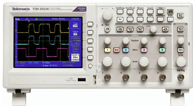
Time is displayed along the X (horizontal) axis, from left to right, and the voltage level of the signal read at each point in time is shown on the Y (vertical) axis.
