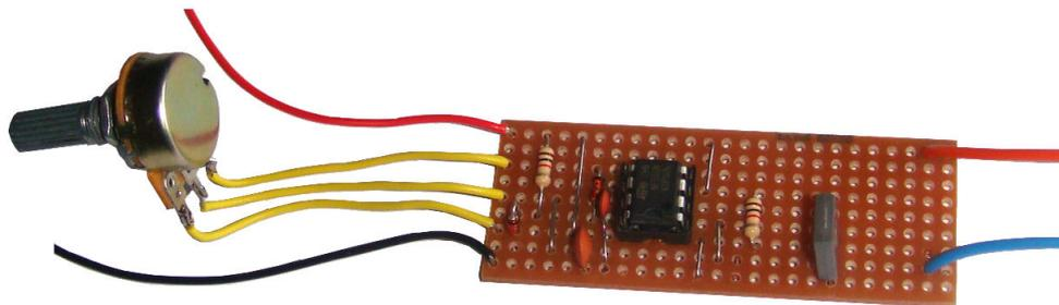
This project can be used to dim a 12V LED strip, as shown in the picture, or dim one or more individual LEDs, using a dropper resistor.
