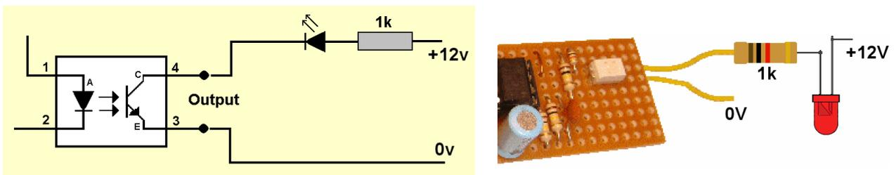
Since the KB814 output is isolated from the rest of the circuit, a separate power supply is needed to provide the 12v that lights the LED.
