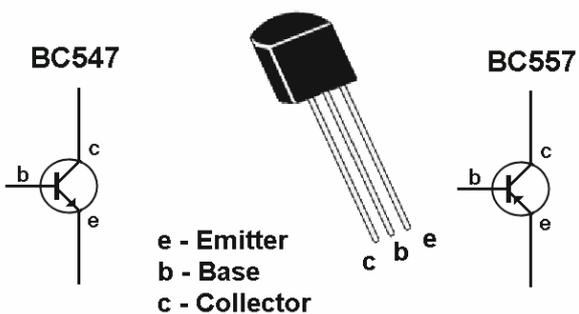
The two transistors use different semiconductor layers in their construction. This means that the BC547 allows current to flow from its collector to emitter when its base is at a higher voltage than its emitter. The BC557 allows current to flow from its emitter to collector when its base is at a lower voltage than its emitter. That's why the red LED lights on 0V while the green LED lights on 5V.
