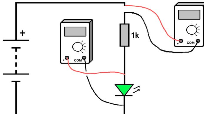
The illustration shows how to measure the voltage across the LED and also the current flowing through the LED. Connecting the meter across the LED tells you what voltage the LED is working on. Connecting the meter in series with the LED tells you what current is flowing through the LED.
