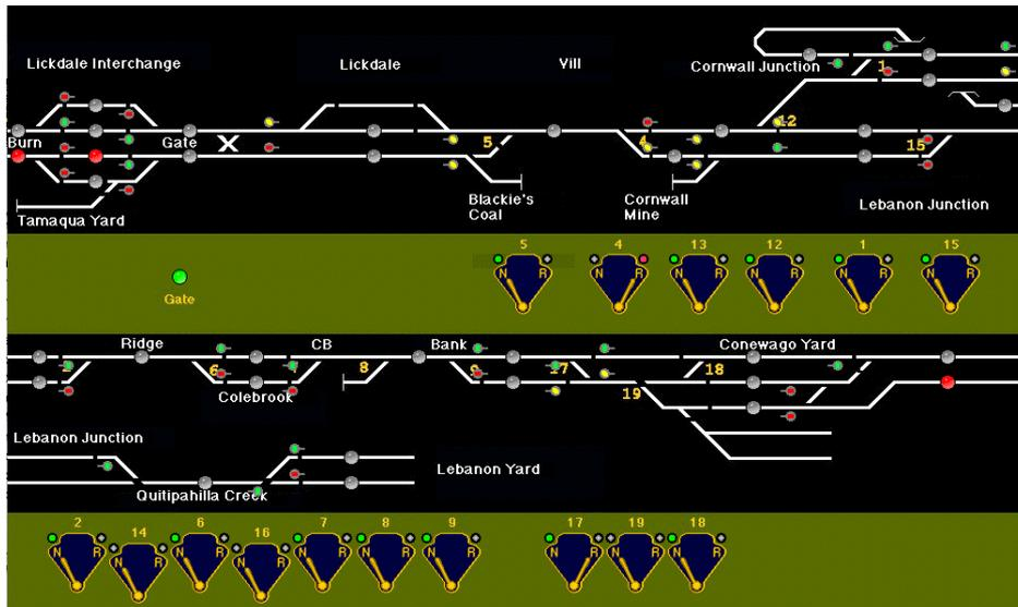
It is an alternative approach to control locos, points, etc. from the screen – or have them run automatically.
