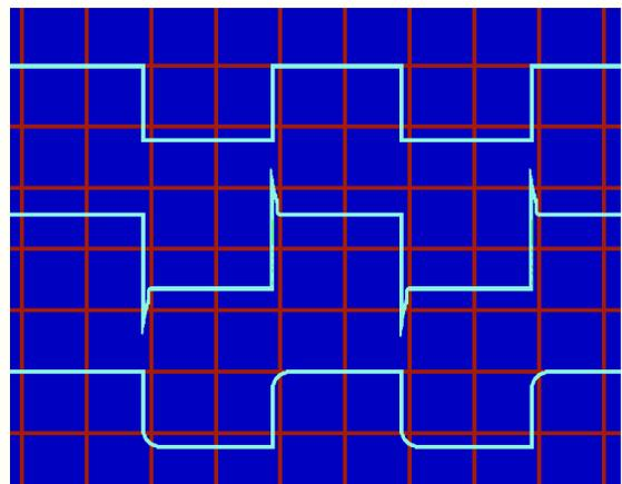
Some signals are entirely cyclic, such as a servo's signal stream or the PWM output from a controller. The exact same waveform is constantly transmitted for any one setting. Change the setting (e.g. increase or decrease the controller's speed) and you get another constantly repeating waveform.
