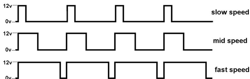
Some DC controllers have a PWM output but don't mention it in their advertisements. You can easily check with an oscilloscope by placing its leads across the controller output and adjusting the horizontal sweep until you see waveforms like those above.
