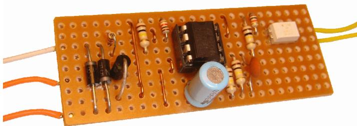
This circuit is only for DCC systems but it will maintain a changed output as long as the train remains in a section of track. Its output is normally at a high resistance but this changes to low resistance when a train sits anywhere on that track section – either moving or stationary.
