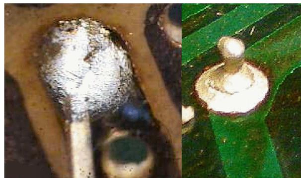
Most dry and disturbed joints are easy to spot on visual inspections. In some other cases, jiggling a component results in one end moving or even lifting from the PCB.
