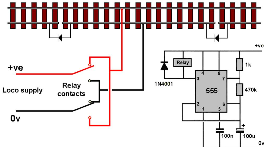
The diagram shows that the track is split into three sections, with a long middle section and a shorter section at each end. The cuts in the track isolate the three sections from each other. One rail is continuous the entire length of the track. The centre section of track is constantly powered from a DC source, while the other sections have a diode wired across the gaps. Being diodes, they only allow current to pass in one direction.
