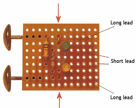
If you have a DCC system, your track voltage is constantly switching polarity at a very fast rate, so both LEDs will light up if DCC power is detected.
