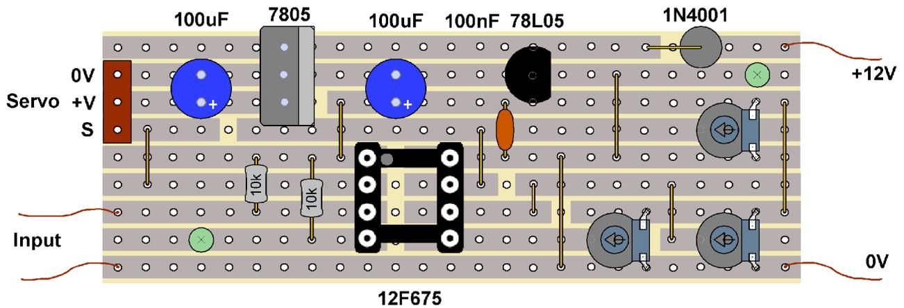
This illustration shows the components and the tracks at the same time. It is really showing where the components should go. It shows the tracks underneath, as if the board was transparent, to help you position the components correctly. If in doubt, consult the earlier photograph.
