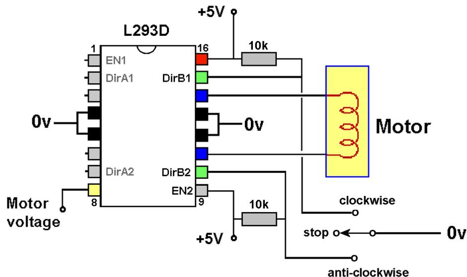
Pin 16, marked in red, is taken to a +5V supply and the pins marked in black are taken to 0V. These supply the power for the IC. The illustrations shows a single motor being controlled.
