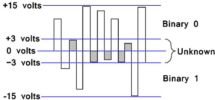
Voltages between +3 volts and -3 volts cannot be converted to known values. These indeterminate values may be caused by interference spikes or may be the result of losses of signal on the line. They are shown shaded in the diagram.
