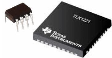
There is a huge range of ICs and each one is designed to carry out a particular function or set of functions. Their internal workings are pre-set at manufacture to carry out specific tasks and these cannot be altered, although their performance can often be tweaked using external components.
