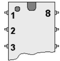
Before connecting power to the circuit, do a close visual inspection of the board, ensuring that you have no short circuits, dry joints, unsoldered connections, etc. Connect the power and check that you read 5V between pins 1 and 8 of the chip.
