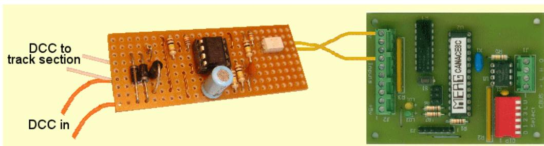
The image shows the detector's output across the CANACE8C's 0v line and input 6. The CANACE8C will send out a message when the train enters the track section and another message when the train leaves.
