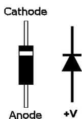
Lastly, the LED and its 1k resistor can be replaced by a 12v relay, if required. You can connect the relay's coil either way round, although the diode (a 1N4001 type is sufficient) has to be wired the correct way round, as in these diagrams.
