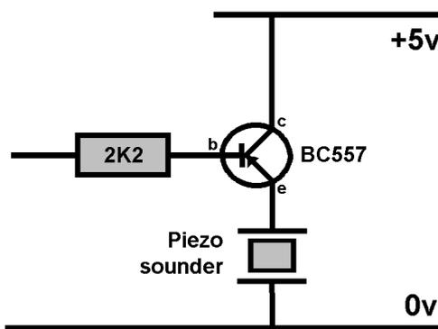
If your module's output can handle that amount of current, you can connect the buzzer directly to the output pin. When a DC voltage is applied across it, it will emit a continuous high pitched tone.
