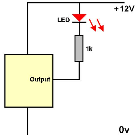
This circuit is an example of '*sinking output*'. The load (LED and resistor) are provided with a high voltage from the positive supply, while the output provides a path for the current to flow to 0V. In effect, the module's output pin has '*sunk*' to the level of 0V.
