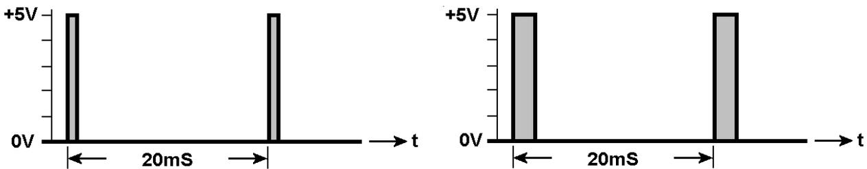
If the sweep speed was set to 1mS/div, you would see 50 pulses on the display but the pulse widths would be so narrow that you would not be able to see the pulse width changing when the servo settings were altered. Its a matter of matching the sweep width to the signal being examined. Oscilloscopes typically handle waveforms from as low as 1Hz up to several MHz, or if you pay a lot more they can cover several hundred GHz.
