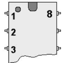
Before connecting power to the circuit, do a close visual inspection of the board, ensuring that you have no short circuits, dry joints, unsoldered connections, etc. Connect the power and check that you read 5V between pins 1 and 8 of the chip.
