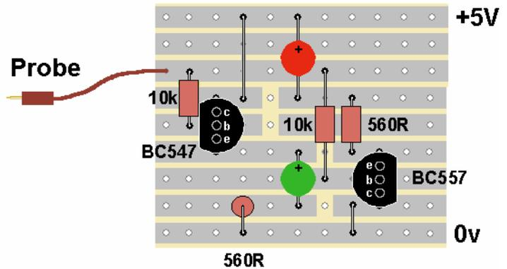
The first step is to cut four breaks in the track at the points shown in the illustration.
