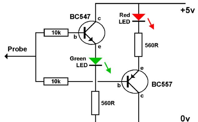
a higher voltage than its emitter. The BC557 is a PNP and allows current to flow from its emitter to collector when its base is at a lower voltage than its emitter. That's why the red LED lights on 0V while the green LED lights on 5V.
