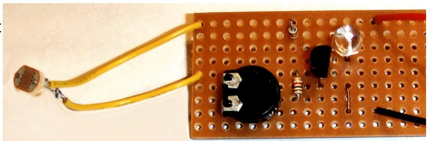
on it. The one shown has a resistance of between 8kohms and 24kohms when exposed to light (at 10 lux), rising to 1Mohm when in darkness. It will have resistance values between those two extremes, as the light value alters.
