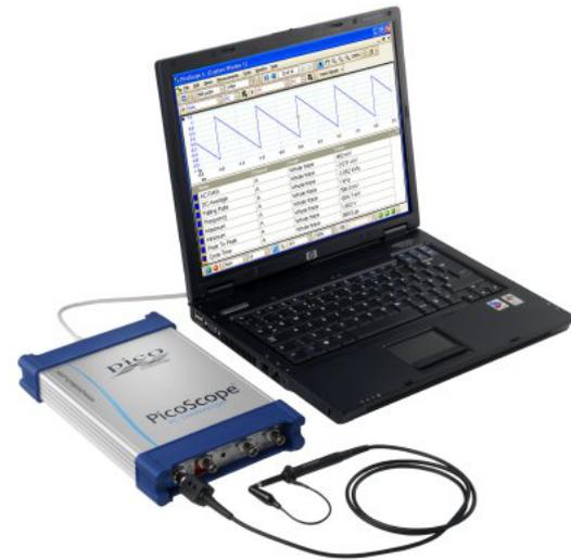
This image shows a PicoScope unit converting a laptop into a temporary oscilloscope.
