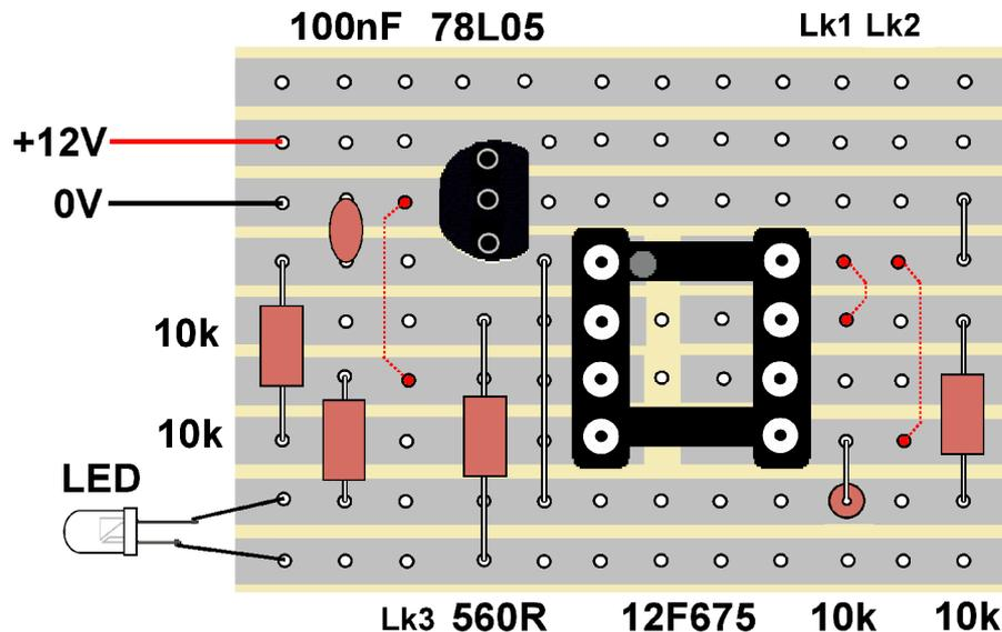
Tip: If you are not too sure, count along the rows and columns on the component side, then poke a wire through the hole where the track is to be cut. Then turn the board over and cut where the wire pokes through.
