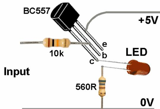
If you intend to illuminate a very high power LED or a LED strip that contains multiple LEDs, you need to use a transistor that can handle these larger currents.
