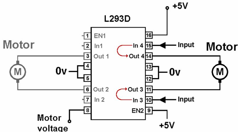
The two chips have identical pin connections and work in exactly the same way. The only real difference is that the L293D can handle 600mA continuously, while the SN754410 can handle 1A continuously (both can handle double these currents for short periods).
