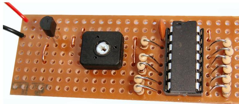
The module has a preset potentiometer that can be adjusted with a small screwdriver. This sets the speed at which lights may be changed. For instance, you may use the shortest delays to test that all the LEDs work. Short delays are also useful at exhibitions, where kids expect things to happen quickly. At other times, you can adjust the delay to your own needs.
