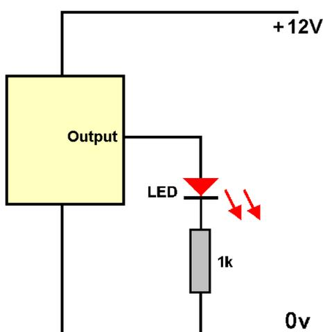
This illustration shows the LED being wired to 0V.
