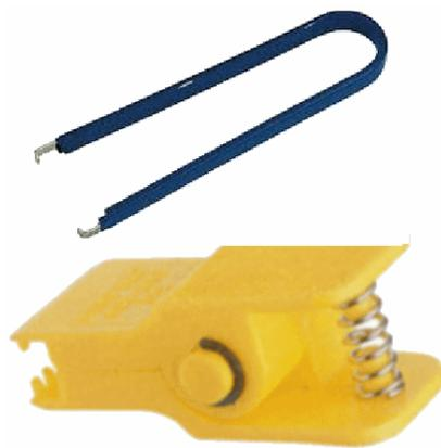
It is also difficult to remove a chip from its socket. Levering it out with a screwdriver, for example, will often bend or break the pins.
