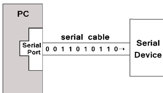
Modern computers pass data between computers and peripherals using one of a number of different serial types of connection. Serial systems are used for keyboards, mice, memory sticks, scanners, digital cameras, broadband routers and modems, local area networks, etc. Example interfaces are the serial port. USB, Firewire, external SATA ports, Bluetooth, IrDA, etc.
