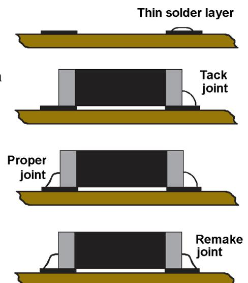
You do not need a lot of solder to make a good joint. If a pad is pre-tinned, you may only need apply a little solder to the iron's tip and apply it to the joint, specially if you apply flux to the pads.
