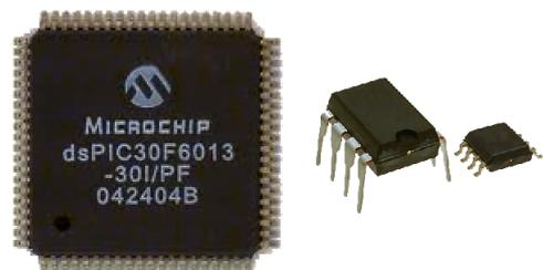
PICs are available in sizes from 6 pins to 144 pins, in either QFN (Quad Flat No Leads), DIL or surface mount pin formats.
