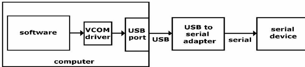
The illustration shows the steps involved in using a serial device (e.g. Servo4 module) on a modern computer that only has USB ports.
