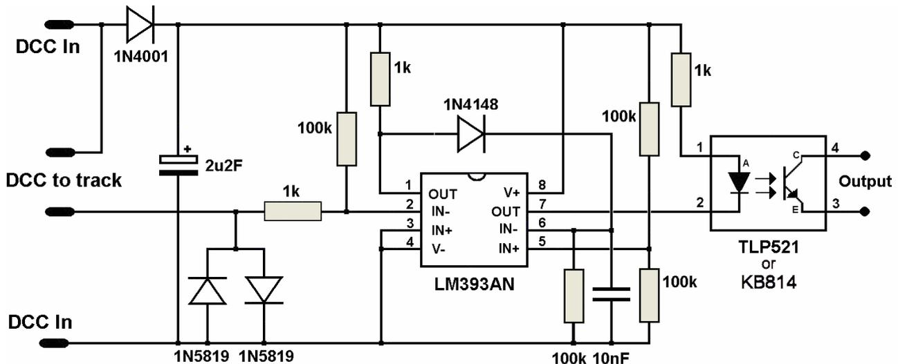
The voltage from a DCC command station alternately swings positive then negative, in what is described as '*bipolar DC*'. The 1N4001 diode only passes the positive-going pulses which are then smoothed out by the 2.2uF (2u2F) capacitor. The voltage across this capacitor provides the DC supply for rest of the circuit.
