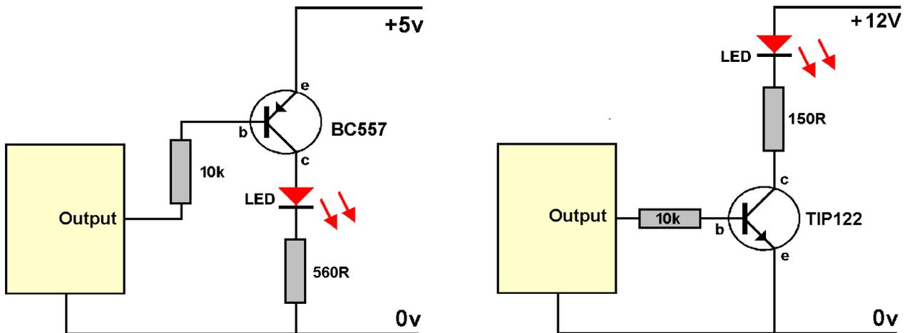
The one on the left uses a transistor as a switch for currents up to 100mA, the maximum that the transistor can handle.
