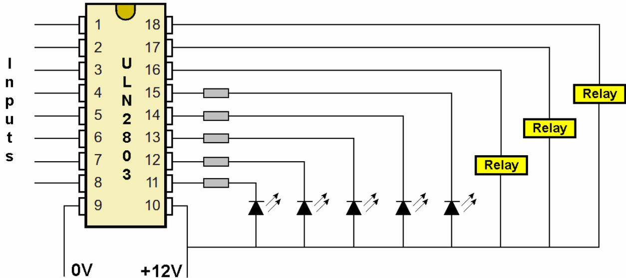
It has two rows of pins and pins 9 and 10 are connected to the power supply.
