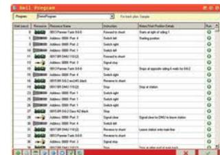
While Hornby's timed list approach is simple to create, it has the serious drawback that it cannot cope with unexpected events such as stalling or derailments. The program
