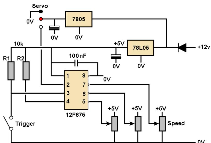
12V supply to the +5V used by the PIC. Another 5V regulator, the 7805, provides a separate +5V line to the servo.
