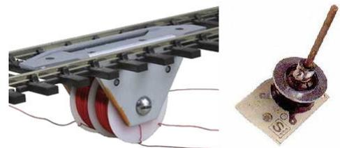
Kadee recommend a 16V DC supply of at least 3A to power their uncoupler. The Seep EM1 model takes 1A at 12V DC and 1.5A at 18V DC. They can both be operated by a simple pushbutton of suitable current rating (check before you fit). Do not use a switch as it may be left on by mistake and overheat until the coil is burn out. Kadee recommend a maximum of two minutes continuous use, although users recommend a much shorter time.
