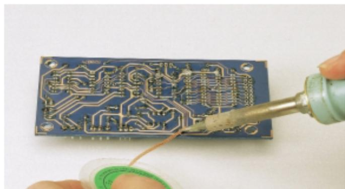
and the soldering iron's tip is then held against the braid.
