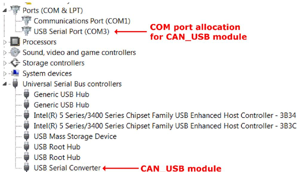
In this example, COM3 has been automatically allocated to the module and this value is the one to enter into any application software when prompted for the COM port number.
