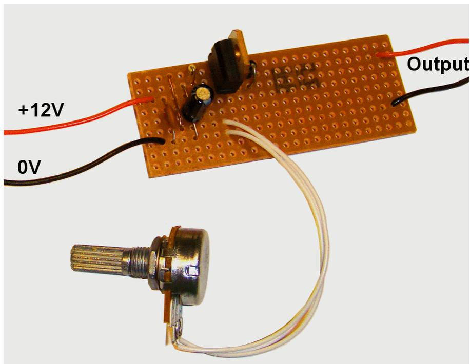
The image shows a variable resistor fitted. This allows easy control over the output voltage, using a knob.
