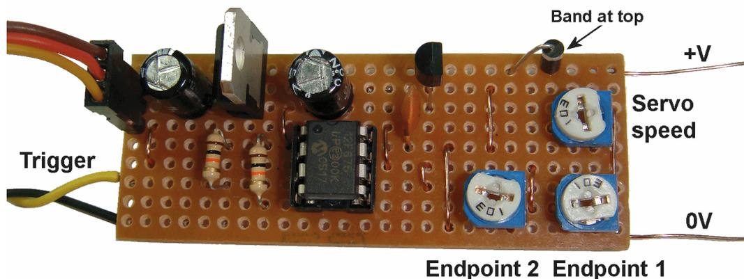
Servos are becoming increasingly popular as a means of operating points. They avoid the thump-thump of solenoid actuators, which require large pulses of current and which can eventually loosen points. Motorised point motors, such as the Tortoise, avoid these problems and produce a slow movement of the point's tie bar. However, they are expensive and require to be manually adjusted.
