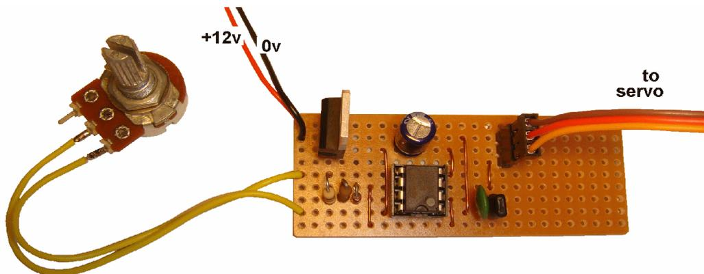
Turning the spindle of the variable resistor (called a '*potentiometer*' or '*pot*') rotates the servo arm. You can turn the pot really slowly, or as fast as you want; the servo will respond accordingly.
