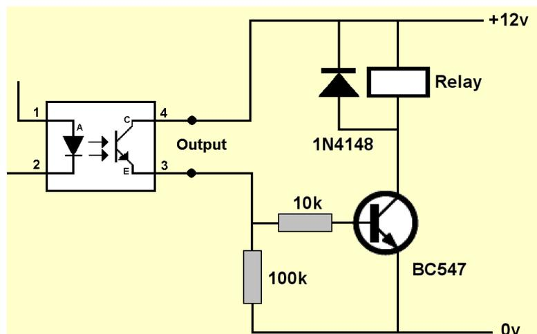
easily-obtained components (the relay and the transistor are available from the Kit Locker). With a bit of repositioning, you could fit most of the parts on
