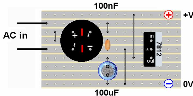
This illustration shows the components and the tracks at the same time. It is really showing where the components should go. It shows the tracks underneath, as if the board was transparent, to help you cut the tracks in the correct places and position the components correctly.
