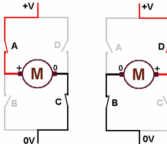
When switches A and C are closed, the motor has a positive potential on its left hand connection and 0v on it other connection. The motor will turn in one direction.
