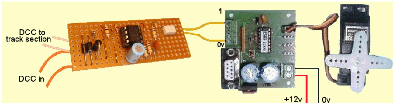
The image shows how the detector's output connects across the Servo4's 0v terminal and the input that you choose to switch (in this case input 1). As simple as that. When the track section is entered, the loco is detected, the TPL521's resistance drops and the servo moves to the new pre-set position. When the loco leaves the section, the resistance increase once more and the servo returns to its previous pre-set position.
