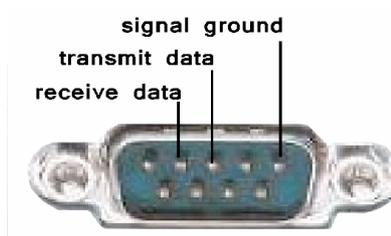
As the illustration shows, one of the pins ('signal ground') is used as a common return for all connections on the port. The data signals are measured with respect to this pin. One pin is used for transmitting data down the serial cable, while another is used to receive data that has been sent to the computer. The other pins are used for various signalling purposes.
