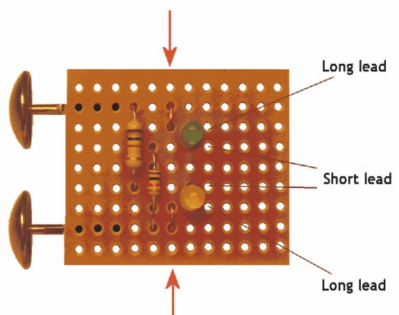
You will notice that the two LEDs are wired in different directions from each other. So, if the track voltage is one polarity, one LED lights up. If the track voltage is wired in the opposite polarity, the other LED lights up. That way, you can still test for track power regardless of whether the controller is set to forward or reverse.
