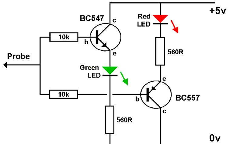
In normal operation, a small increase in current through the transistor's base results in a larger current through its collector. The total resistance of the LED and resistor means that there is a maximum current that can flow through the emitter/collector. When this point is reached, increasing the base current has no further effect. The transistor is said to be in '*saturation*'. The 10k resistors limit the base current to be sufficient to switch the transistor fully saturated.
