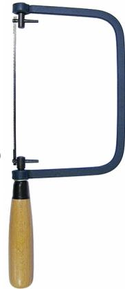
A '*Fret saw*' is like a coping saw with a deeper throat, perhaps 10" or 12". Their blades are not pinned but are clamped at each end of the saw with thumb screws. They use thinner saw blades, allowing them to cut tighter curves than a coping saw and produce more intricate results. The finer blades make them more vulnerable to snapping than coping blades. Also, many users find the larger frame more awkward to work with.
