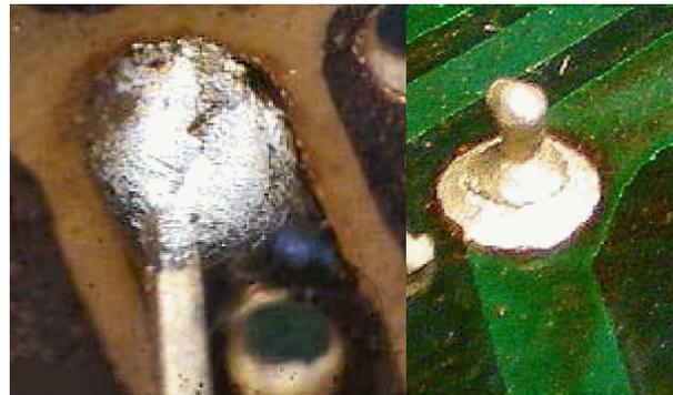
Most dry and disturbed joints are easy to spot on visual inspections. In some other cases, jiggling a component results in one end moving or even lifting from the PCB.
