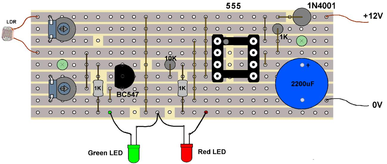
Layout for common anode signals
