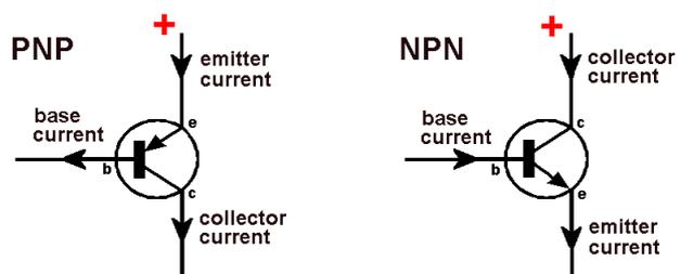
In both cases, the base connection can be thought of as a tap that regulates the amount of current flowing between the other two connections (another type of transistor, the FET, even calls the connections the 'source', the 'gate' and the 'drain').
