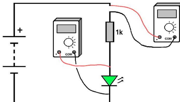
The illustration shows how to measure the voltage across the LED and also the current flowing through the LED. Connecting the meter across the LED tells you what voltage the LED is working on. Connecting the meter in series with the LED tells you what current is flowing through the LED.
