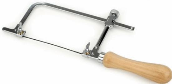
A '*Jewellers Saw*' also has its blades clamped by thumbscrews but its 'C' frame is adjustable. With the other saws, a snapped blade means a discarded blade. With the jeweller's saw, you can still use the remains of a broken blade by adjusting the frame width. Their blades are generally even thinner than those used by fret saws, resulting in even more intricate cuts and a smaller kerf.
