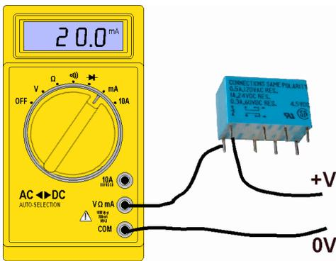
If there is any doubt about the above circuit, you can check what the module's current handling capacity is and compare it with that need to operate your relay. If you are lucky, you will have the relay's specification which will include its coil resistance, allowing you to calculate the expected current for the supply voltage you are using.
