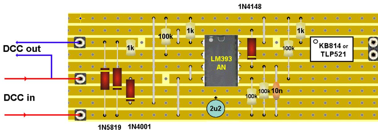
This illustration shows the components and the tracks at the same time. It is really showing where the components should go. It shows the tracks underneath, as if the board was transparent, to help you cut the tracks in the correct places and position the components correctly.
