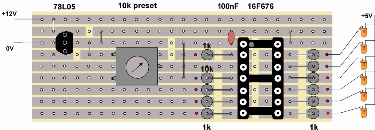
Make sure that you cut tracks where indicated in the above illustration. Check that all 22 are cut and that there are no remaining tiny strips of copper bridging any of the cuts. The next step is to clean the copper strips and component leads prior to soldering.
