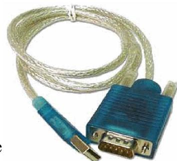
carries out the conversion between USB and serial formats.
