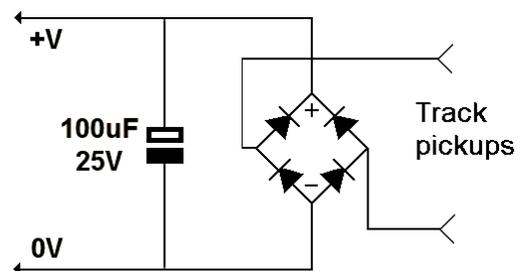
Of course, if you are using DCC, there is continual power to the track pickups and the LED will flash even at slow speeds. Unfortunately, it will also flash when the motor is stationary. However, if you have an unused output from the DCC decoder, such as a headlamp connection, this could provide a switched supply to the flasher module.
