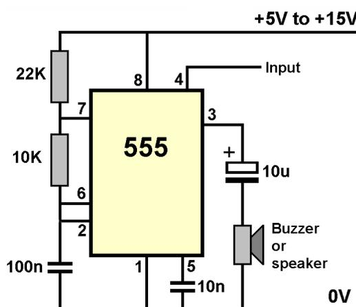
This circuit is a simple oscillator that can be turned on by raising its input pin 4 to the positive supply. While pin 4 is held low, the circuit does not oscillate.
